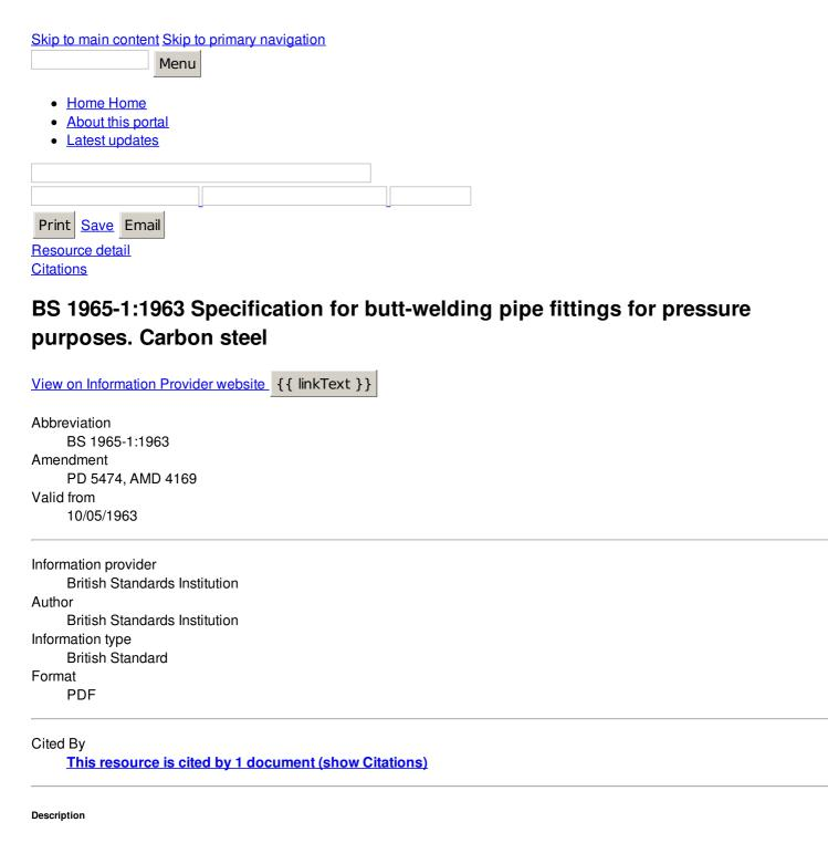
This Standard specifies leading dimensions, tolerances and materials for 90 deg and 45 deg elbows, 180 deg return bends, equal tees, concentric and eccentric reducers and caps, in carbon steel, for butt-welding on to pipes. Details of testing and marking are also given.
