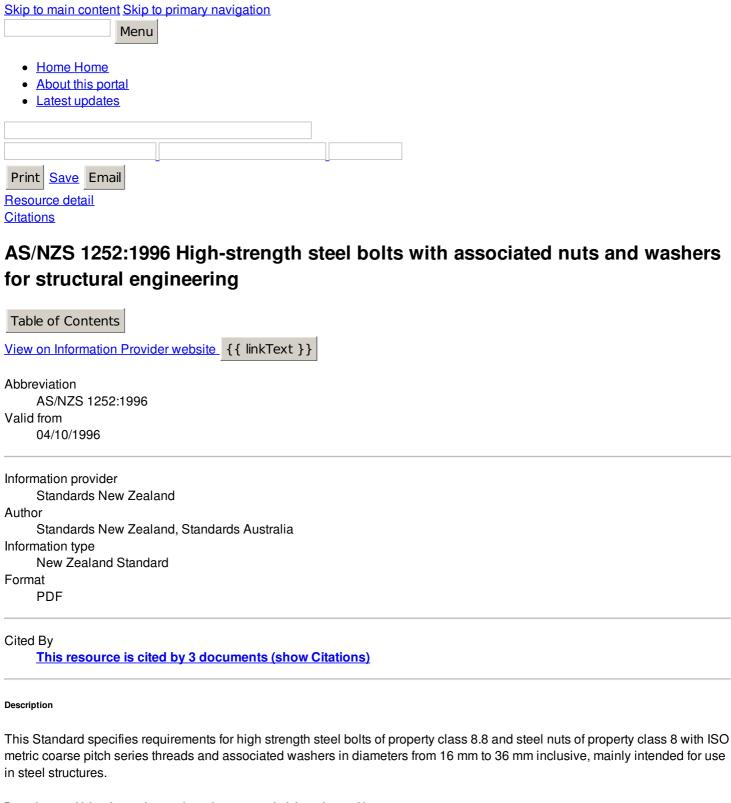
metric coarse pitch series threads and associated washers in diameters from 16 mm to 36 mm inclusive, mainly intended for use
